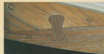
Above, steering quadrant, seacocks and engine exhaust hosing in place. Left, butterfly scarf helps to secure the teak toerail
