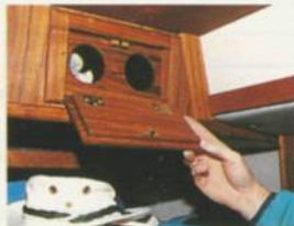
Customised accommodation aboard the 37. The tubular stowage (above) is for charts, which would be better off flat
