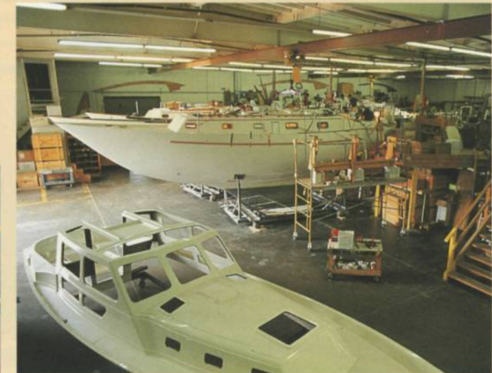
Left, the accommodation close to completion. Above, the new pilothouse version of the 32 deck moulding in the fitting-out bay
