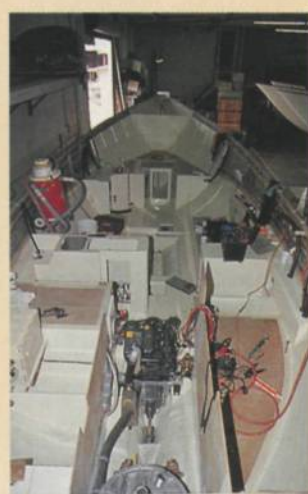
Right, engine installation, plumbing and wiring are all thoroughly checked while they are still accessible. Far right, preparing to bond the teak toerail to the bulwarks. Teak decks are an option
