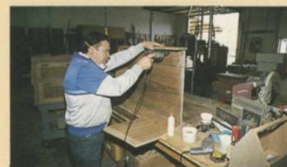
Above and below, constructing furniture outside the yacht and then installing it
