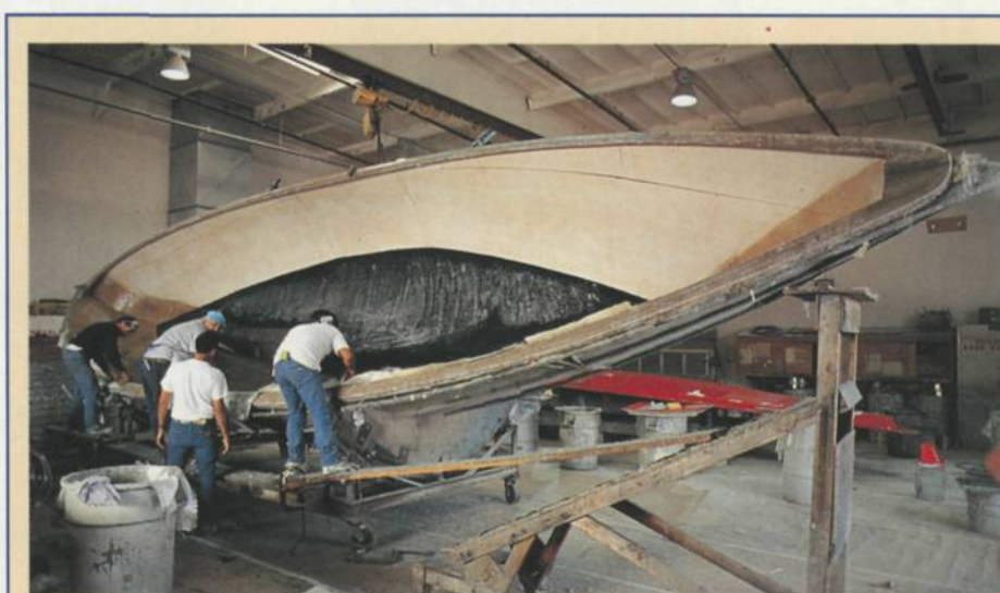
Above, the Californian climate allows moulding to take place in open-sided sheds. Right, with liners in place, the 37 is almost ready to receive furniture, which has been built in the wood-working shop. Note the topsides-mounted chainplates
