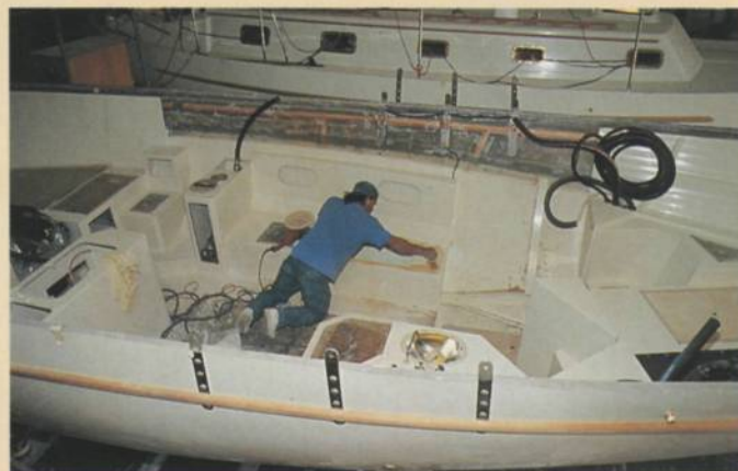
Above, the Californian climate allows moulding to take place in open-sided sheds. Right, with liners in place, the 37 is almost ready to receive furniture, which has been built in the wood-working shop. Note the topsides-mounted chainplates
