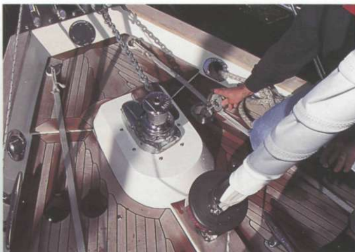
An organised foredeck, but the secondary rode is on the wrong side for this windlass
