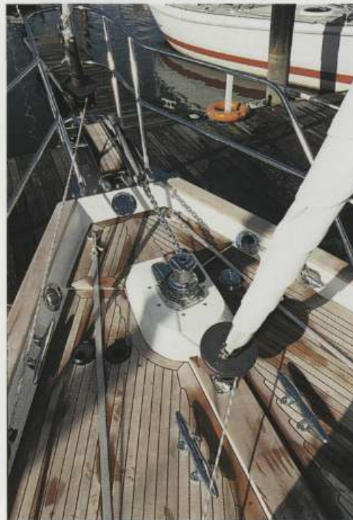
The enclosed G-shaped galley (above, left) offers a safe refuge for the cook in most offshore conditions. Placing the mainsheet track (above) forward of the sprayhood keeps the cockpit clear. The foredeck set-up, with twin anchor rollers in a plank bowsprit, is excellent for blue water cruising
