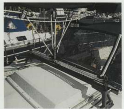
The enclosed G-shaped galley (above, left) offers a safe refuge for the cook in most offshore conditions. Placing the mainsheet track (above) forward of the sprayhood keeps the cockpit clear. The foredeck set-up, with twin anchor rollers in a plank bowsprit, is excellent for blue water cruising
