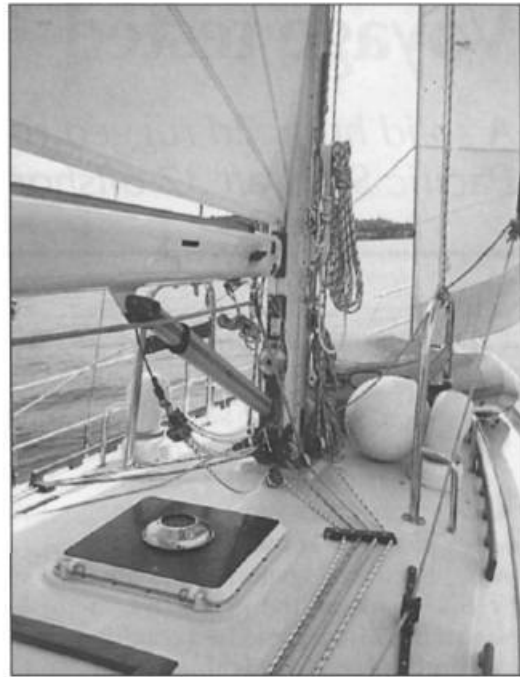
A vang supports the boom, eliminating a topping lift. The mainsail furling system includes a low-profile winch beneath the boom. Thus the main can be furled both at the mast and in the cockpit.
