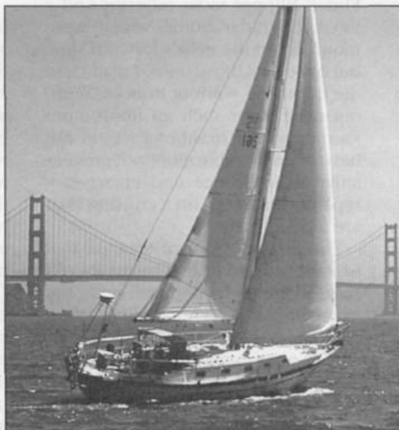
With its canoe stern, modest beam, and symmetrical hull, the Pacific Seacraft 37 tracks well, allowing the boat to be easily steered by windvane or autopilot. A rugged mast, with shrouds leading out to the gunwhales, supports a powerful cutter rig, ideal for both upwind and off-the-wind sailing.
