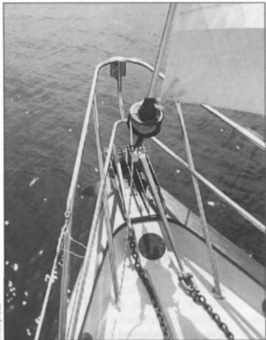
A pair of bow rollers are standard on the Pacific Seacraft. With this setup one can stream twin anchors and rode when needed. Increased bow volume above the waterline adds reserve buoyancy.
